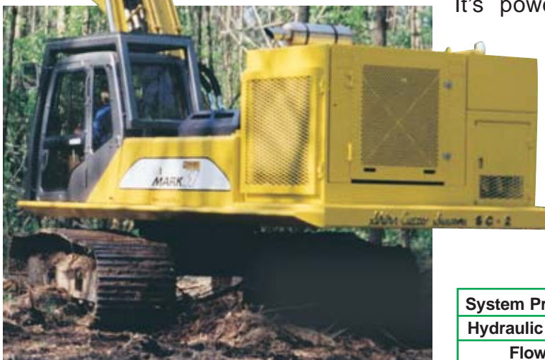
Kobelco 220 with Seppi Forest DT-150 cutting head and Shinn SC-2 hydraulic power pack. Complete system weighs approximately 66,000 lbs.
