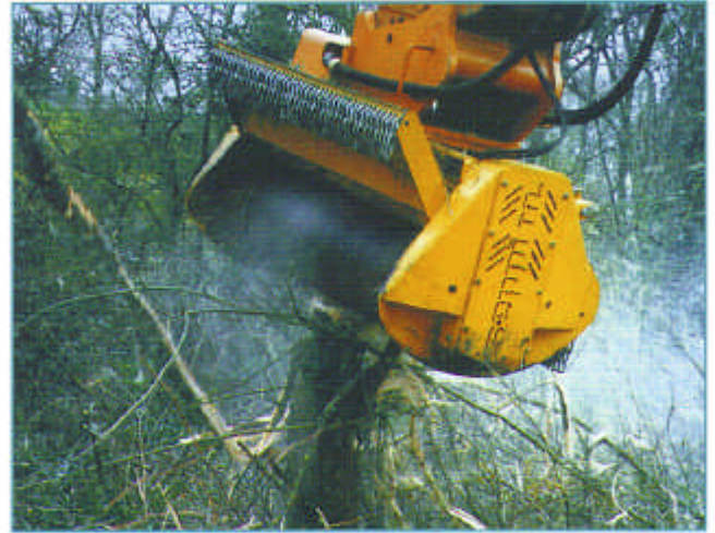
The forestry rotor allows the grinding of tree trunks
